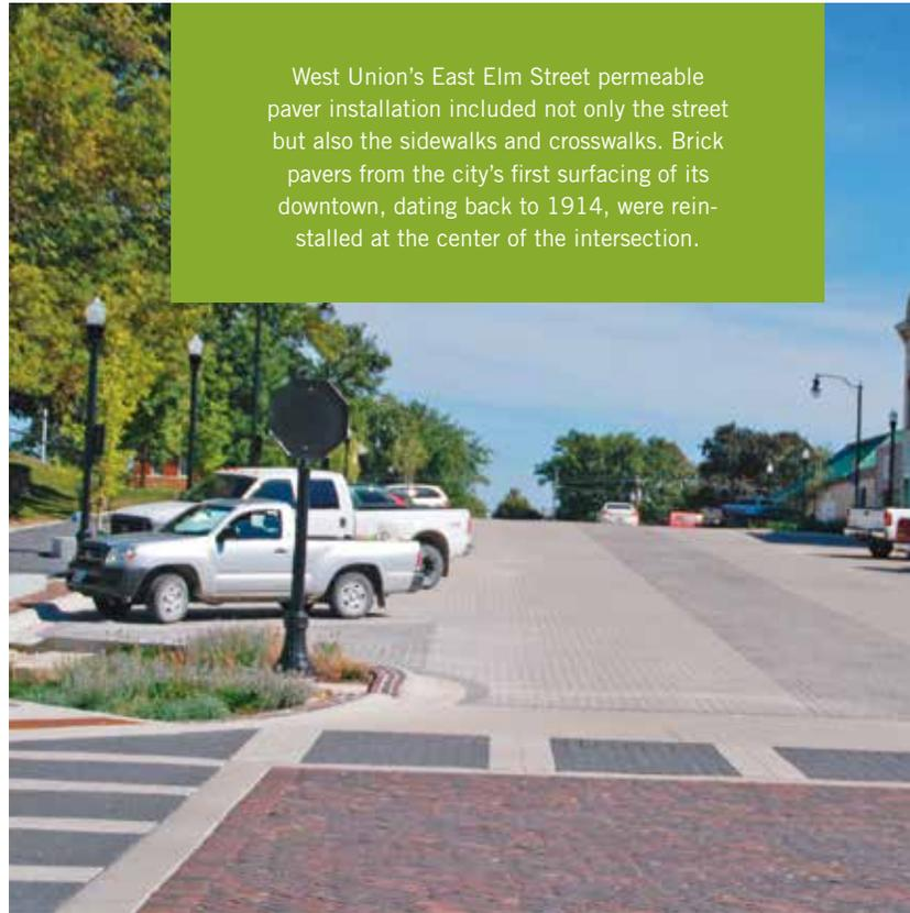
West Union's East Elm Street permeable paver installation included not only the street but also the sidewalks and crosswalks. Brick pavers from the city's first surfacing of its downtown, dating back to 1914, were reinstalled at the center of the intersection.
